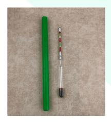
Alcoholmeter Hydrometers, Tripple Scale
